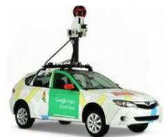
The fish eye lens camera takes pictures every hundred feet or so. If you have seen pictures taken with a fish eye lens, you know that they are very distorted. The software in Google Street Views provides for real time distortion removal. This means that as you pan around and up and down on a street view image the picture looks normal.
