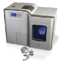
The end result of 3D printing is a part or assembly of parts that are made directly from models designed with computer software. Once the 3D data base has been created, the data is sent to a machine that build up a part by adding thin layers until the part is complete.
